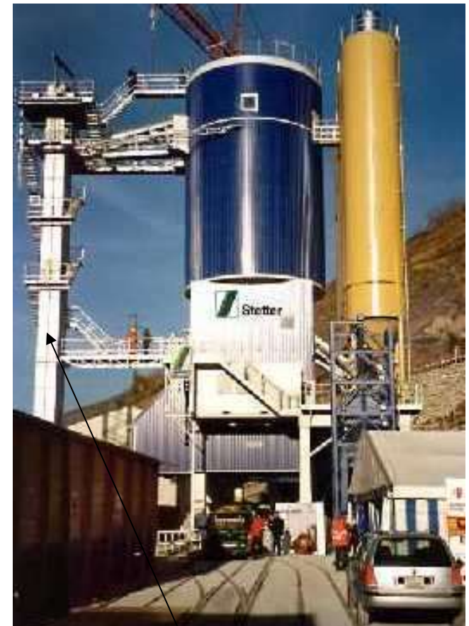
Vertical Bucket Elevator (rarely used for aggregate)
