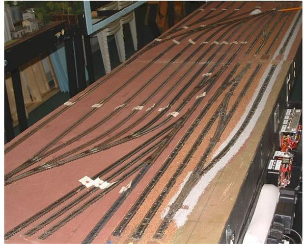
Lee has re-configured the power controls and done some rewiring so that now they can run DC or DCC on any track, with the throw of a toggle switch on the panel. This panel can be removed for travel fairly easily.
